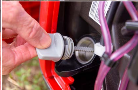
Left: Draining the oil Right: Removing the front panel of the generator Bottom right: Oil dipstick
