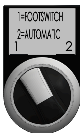
Figure 20: Automatic lid switch
