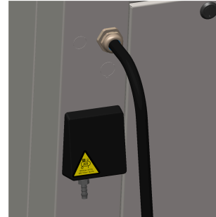
Figure 7: Hose connection for compressed air
